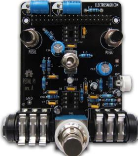
In this step it is important to solder the remaining parts from small to big, the optimum order is:
