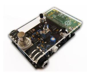
Finally the plastic cover can be placed, it is kept in placed by the foot-switch nut & plastic washer and two M2.5x25 screws & nuts.
