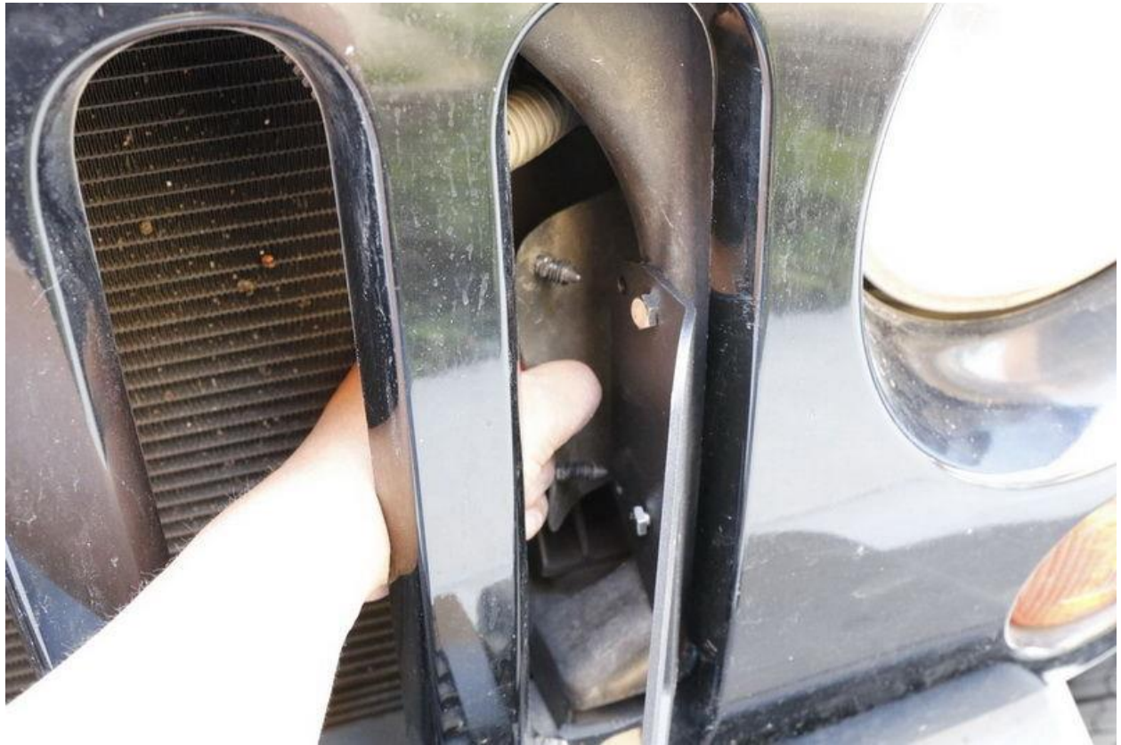
Step 4: Clip the plastic fasteners into the outer holes of the mounting brackets for the light bar.
