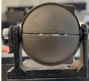
3. Turn the system on and allow the eyes to blink a couple of times. This will set the correct positioning of the eyelids during blinking and eyes during x-axis motion. **(Note: If you hear the servo gears grinding or the eye movement doesn't seem natural, you may need to change the angles of the servo motion to accommodate your setup.)**
