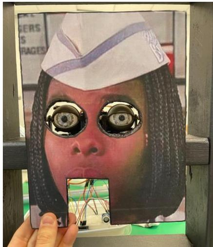
3. Place the eye mechanism on the middle shelf of the supporting structure and align it with the face in a location that lines up with the eye cutouts of the face. ***(Note: Be sure to offset the location of the eye mechanism behind the face to ensure the servo arm or eyelids contact the back of the face cardboard.)***
