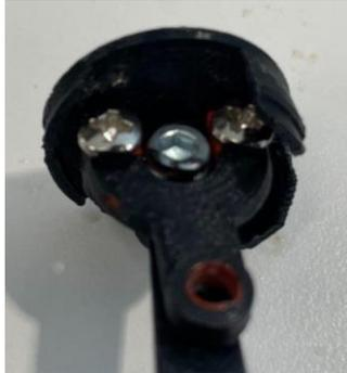
5. Attach the servo arm on the final hole to the center of the three-point connector using a 5mm M3 bolt. **(Note: The hole on the servo arm will need to be drilled out to 2.5-2.8 mm to accept the screw.)**
