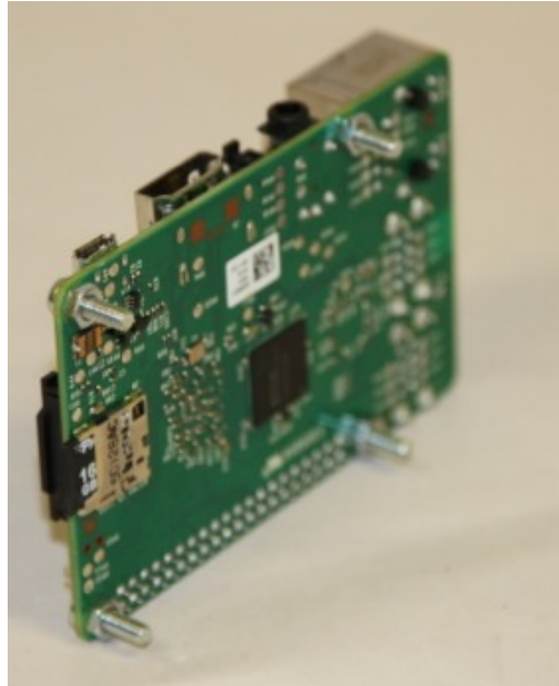
Raspberry Pi Board with mounting bolts attached and nuts underside
