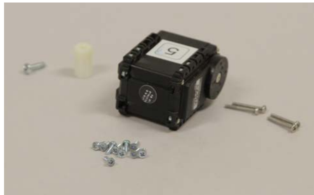
Servo 5 connecting details with spacer for Left Hand Side
