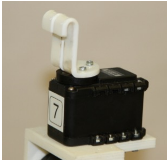
Camera plate attached to Servo 7
