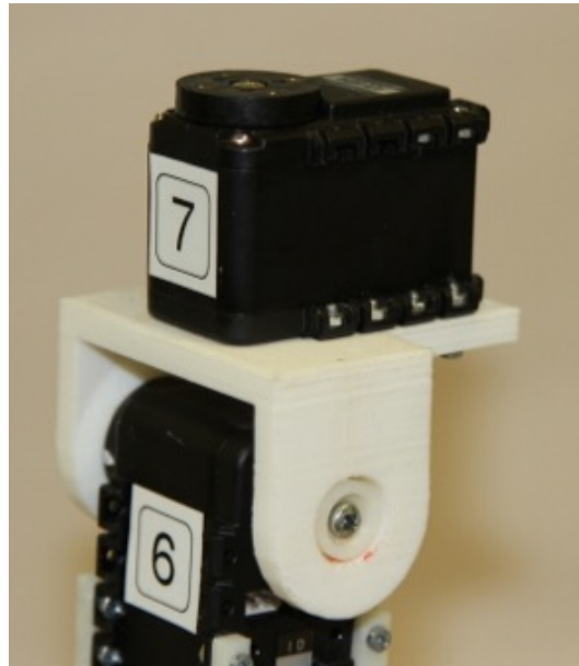
Camera mount attached to Servo 6
