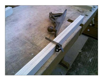
Step #4: Square one edge to the board's surface. Use a jointer to make the edge square to the face of the board. Use a square to ensure that the edge is 90 degrees to the face.
