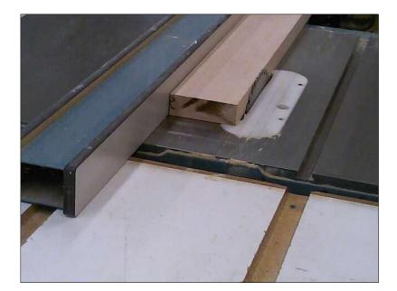
Step #5: Use a table saw to create parallel edges.
