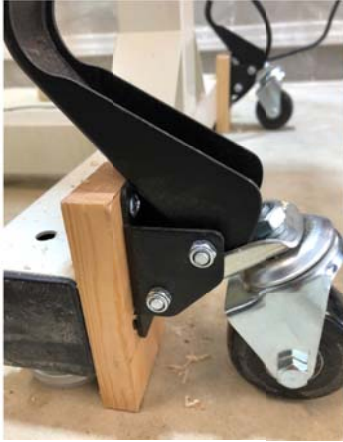
With wood brace
