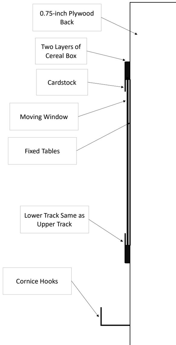
Figure 9: Edge view of simple to build keyholder
