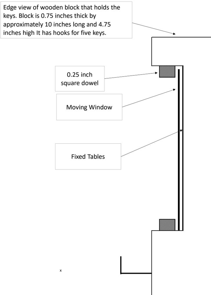
Figure 4: Edge view of fist prototype
