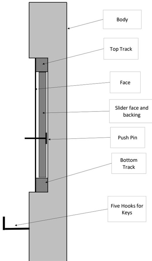
Figure 6: Edge view of keyholder with a moving slider calendar
