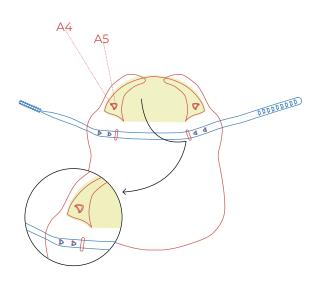
Bend **A5** to clip into **A4**. Ensure the inner flap (marked in yellow) sits on top of the exterior flaps.
