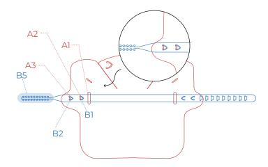
Thread **B5** through **A1**, clip **B2** into **A3** and **B1** into **A2**. Pull to seat both tags securely.
