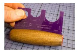
The length of the gauge is 90mm so it can be used to mark the lines for the parting tool and the width is 45mm so the middle can be found.
