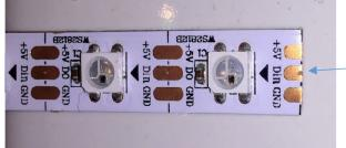
The LED strips have pads you can solder to. +5 & Gnd for the power and the Din and Dout (DO) for the data. The array of RGB data passes along the LEDs, and each LED takes its value and passes the rest down the chain.
