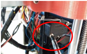
Fig 6: Tighten up Z-axis limit switch
