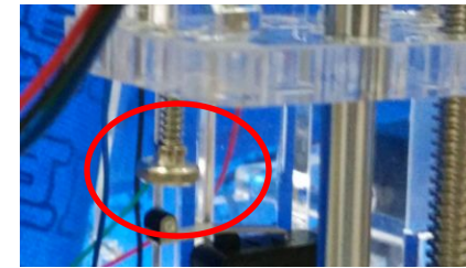
Fig 7: Adjust screw of Z offset
