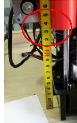
Fig 4: measure height of X-slide
