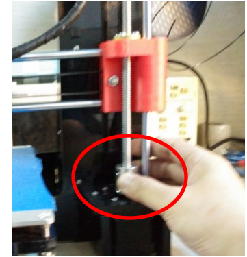
Fig 5: Adjust X-slide height
