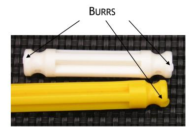
You may think that the odd burr doesn't matter, but if you connect one of the damaged rods to a connector, there is a good chance that the rod and the connector won't lie in a straight line. Also, it won't have the strength of a proper connection.
