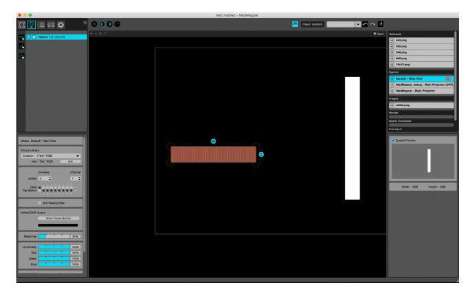
Don't change « universe » and « channel ». Universe 0 is the one sent to the teensy and channel 1 is the first channel that will control LEDs (see step 5)
