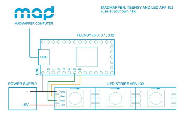
The data pin, and the eventual clock pin, must be connected to digital pins on the teensy.
