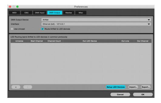
There is a table showing up below. Just press the + button on the bottom left, a new line will appear. Each line will allow sending a part of an ArtNet universe data to a LED device. Actually supported LED devices are : teensy (with MadLED protocol), arduino (with MadLED protocol) and BlinkyTile / BlinkyTape devices.
