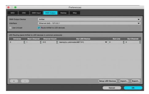
With this setup, MadMapper will forward ArtNet universe 0 data (channels 1 to 512, so the whole universe), to the teensy at channel 0. You could use ArtNet universe 1 to feed channels 512-1023 of the teensy.
