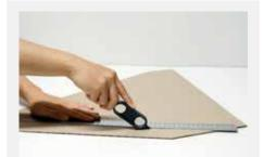
To crease the cardboard on the fold lines, lightly score it with the tip end of the Safe-Saw.
