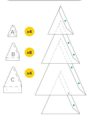
Use the templates on the right to measure and cut the panels. Note how many you need of each panel above.
