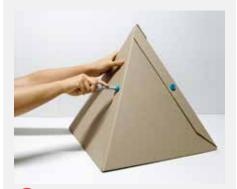
Each module uses four identical triangle panels. Place the flap of one triangle over the edge of the second and align the holes. Screw in place.
