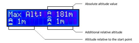
Switch to the maximal altitudes screen by short pressing "Button 3" in the "Main screen". Zeroing of the maximal altitudes can be done by long pressing "Button 3".
