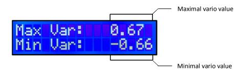
Switching to the MAX/MIN variometer value screen is made by short pressing "Button 3" in the "Max altitudes screen".
