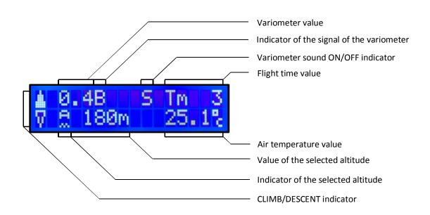
In this case, read the screen values as follows: the aircraft is climbing with vario value +0.4 m/s, the vario signal is active, the buzzer is switched on, the flight time is 3 minutes, the selected absolute altitude is 180 meters, the air temperature is +25.1 degrees.
