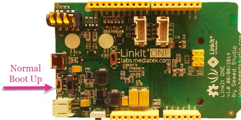
*Figure 12 Normal boot up switch mode on the LinkIt ONE development board*
