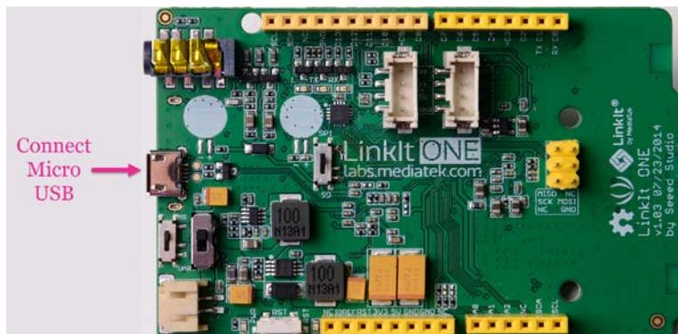
*Figure 8 Micro USB connector on the LinkIt ONE development board*
