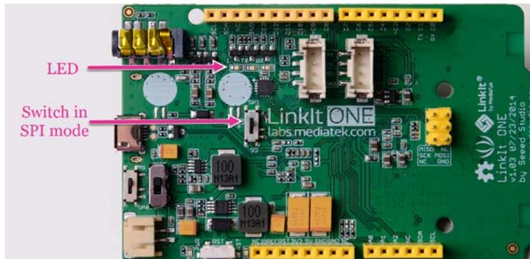
Figure 16 The LED on the LinkIt ONE board
