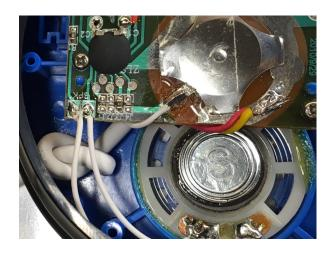
Tie a knot in your cable so that it will not be pulled out. Route your wires carefully and out of the way. When you test the button, make sure it feels the same as when you started. Also try spinning the cover around until it "sits" in place.
