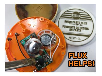
The acid in the flux makes for a much easier time when it comes to soldering.
