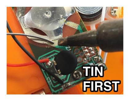
Work the solder in until it catches nicely on the circuit trace.
