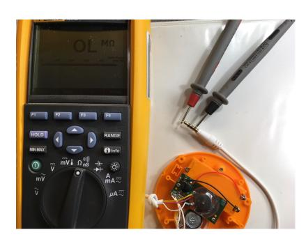
Ring out your work to check that your switch is closing correctly, do this by pressing on the push button while checking with your multimeter for a good connection. You should be seeing less than 5 ohms.
