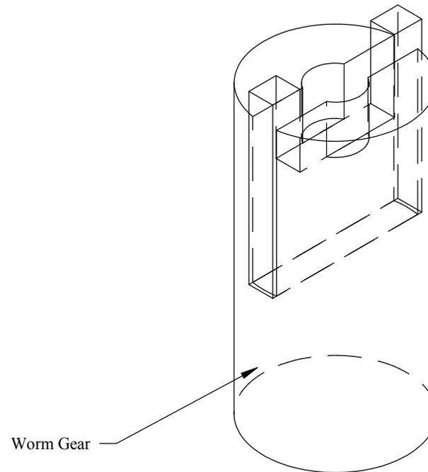
Motor/Worm Gear Adapter
