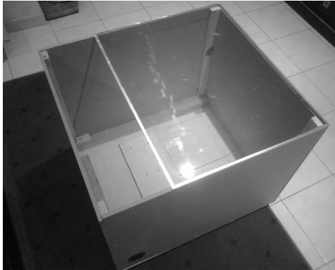
Figure 3: Semi-built box based on 3D model above.
