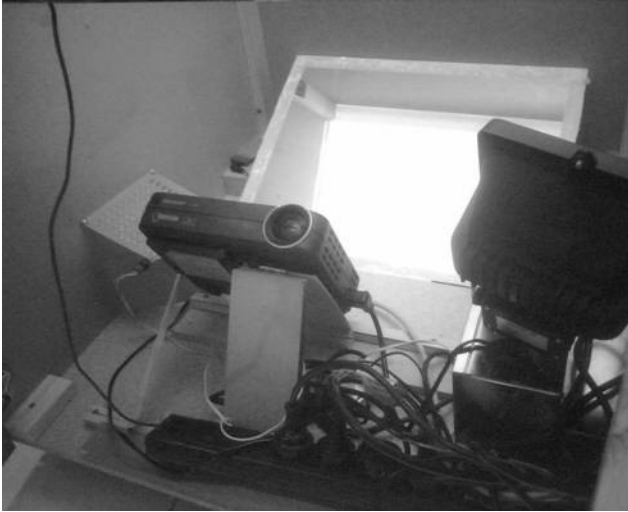
Figure 5: Image of DI setup - projector, illuminators, mirror
