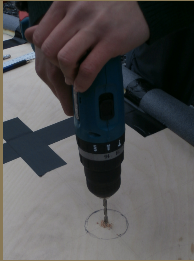
Use a drill to pre-drill a hole for the next step. Use the right drill. (depends on the drill bit)
