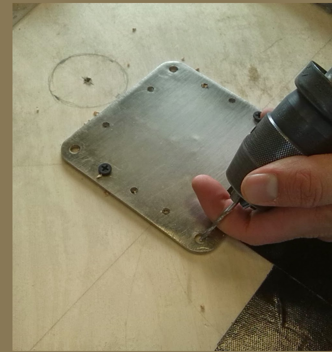
Drill some holes in the (mastfeet). Use the holes to pre-drill new smaller ones.
