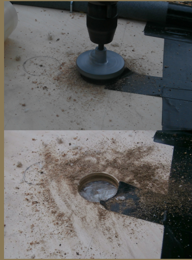
Drill the hole for the mast. Use a drill bit. Use some tape to avoid splinters.
