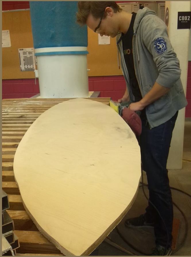
Cut the shape of the surfboard out of multiplex by using a jigsaw. Get rid of bumps by sanding the edges.
