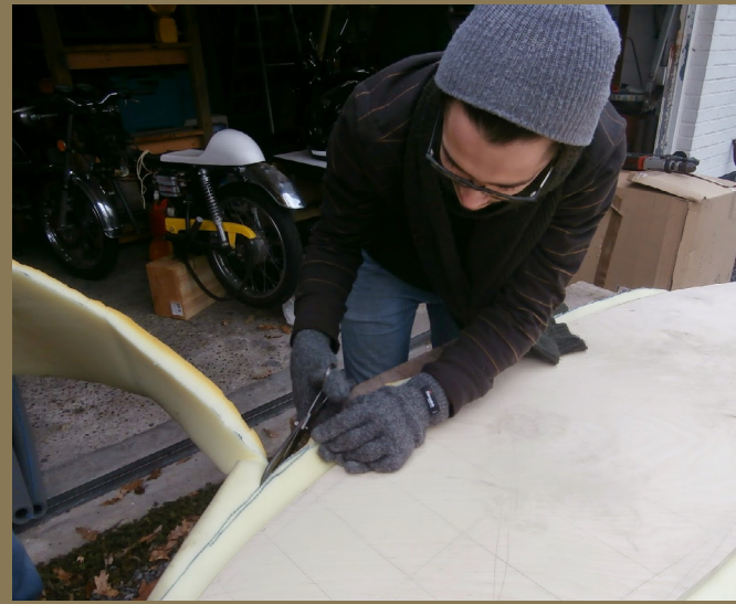
Cut the surfboards shape out of foam. Make sure you have extra space left for the attachment on the board. (oversize the dimensions)
