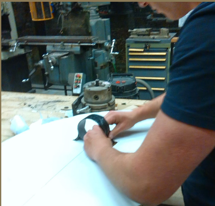
Take the cardboard shapes. Use ductape to attatch a short tube of pvc onto the cardboard.
