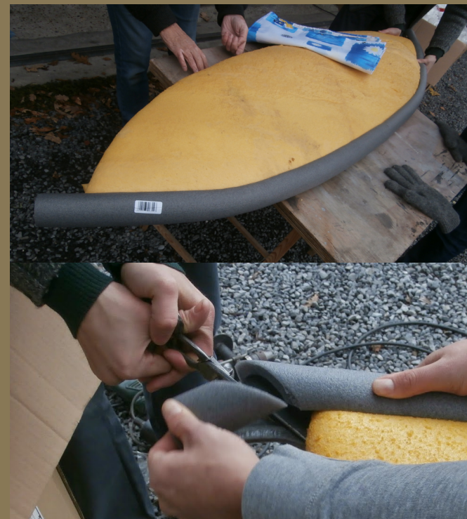
Apply the isolation on to the board. Cut the isolation on the right dimensions.
