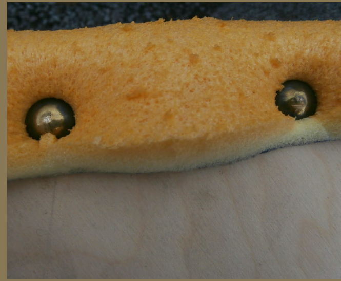
Attach one side of the foam onto the board. Use spikes with a rounded head.
