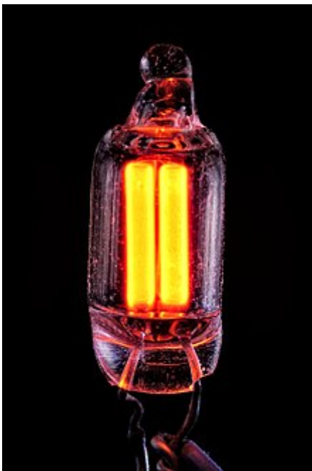
NE-2 type neon lamp powered by alternating current (AC)
