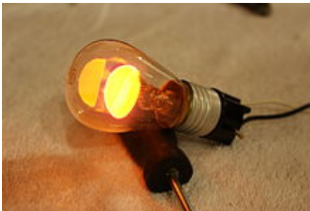
A General Electric NE-34 glow lamp, manufactured circa 1930
