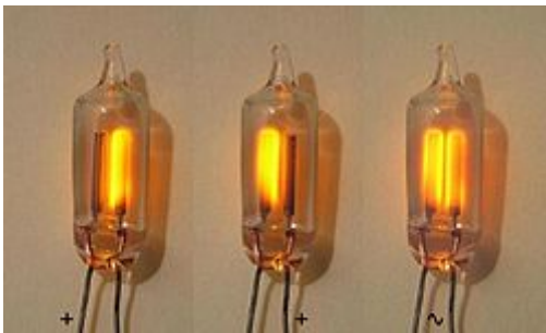
+DC (left), -DC (center), AC (right) supplied to NE-2 type neon lamps
