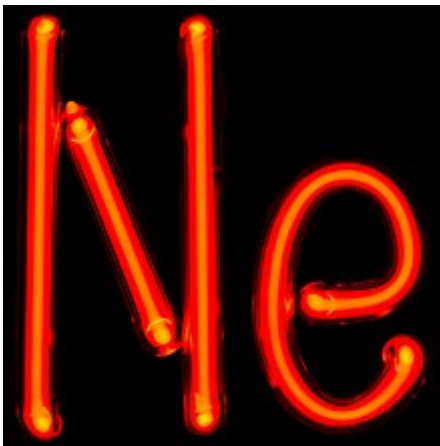
Gas discharge tube containing neon, which was first displayed by Ramsay and Travers; "Ne" is the symbol for neon, one of the chemical elements.
