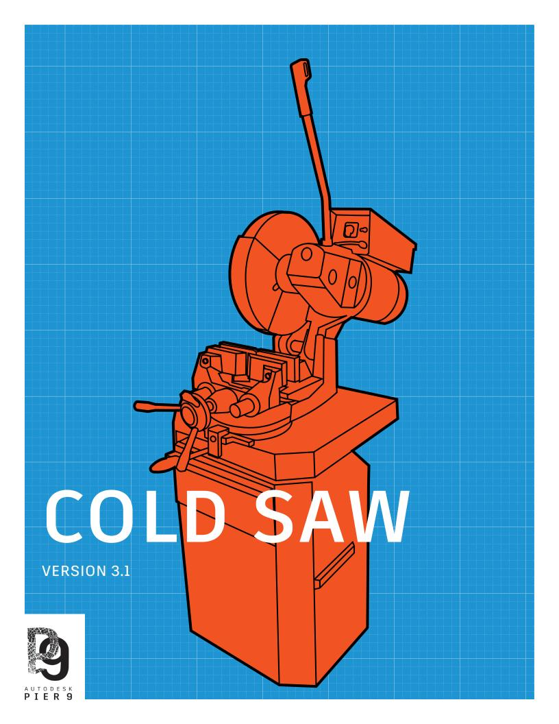
THE COLD SAW MAKES ACCURATE STRAIGHT & MITERED CUTS IN METAL.
