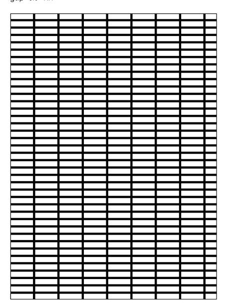
A diagram of the final Running Bond. brick 12x3 mm gap 0.9 mm
