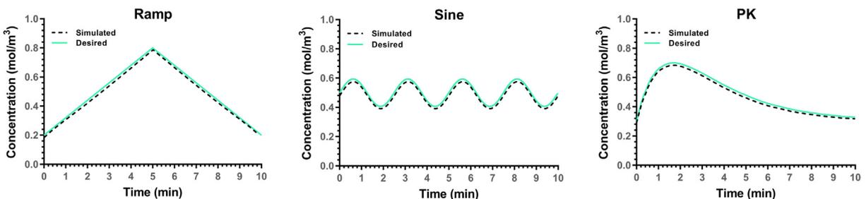
**Fig. 6.** Validation of the flow rate "csv" file to achieve desired concentration using the CFD model. The developed CFD model allows us to computationally validate that our prescribed flow waveforms create the desired concentration profiles, thus minimizing the need for real measurement-based validation before a stimulation experiment.
