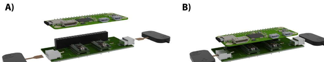
**Fig. 3.** Second step of device assembly. A) Once the components are soldered in you can push in the Raspberry Pi (that already has male headers) and the pumps. B) The system is now ready for software installation.
