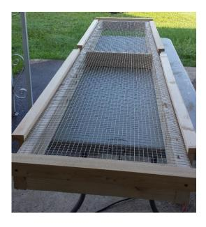
See how the additional pieces form a ridge around the perimeter of the shelf equaling the 22" finished width.
