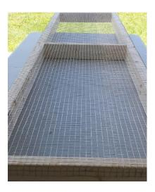
Next I flipped the shelf upside-down with the fabric on the bottom. I used 1x4 pieces under the shelf to allow some finger room for checking the alignment of the 1x4 pieces being attached to the top perimeter of the shelf. I used the 1x4s to additionally secure the hardware fabric AND to protect myself from the overhanging fabric while working in the greenhouse.
