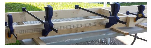
I used scraps of 2x4 to eyeball the position of the longer 1x4 pieces. I cut these to 40" long and screwed them into the sides with the 2" screws. (The scraps simulate the leg placement). On the ends I used 1x4 pieces cut to 22".
