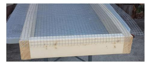
To secure the "fabric" I cut the corners, folded it over the 2x4 frame and used a staple gun. Unfortunately, I still had to use a hammer to push the staples into the wood and in some cases to flatten the fabric to the frame.
