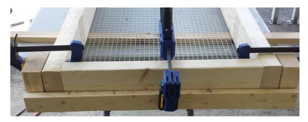
Then I flipped the shelf over (with the fabric side up) to attach additional 1x4 pieces on top of those around the sides. I used my nail gun with 1.25" finish nails for this.
