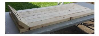
I also attached short 2x4 pieces to the 48" legs to support a shelf I made from a 1x6. The tops of the front legs are flush with the 1x4 perimeter pieces. This also creates a nice lip to prevent anything from falling off the shelves.
