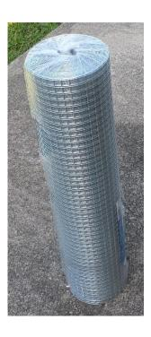
To assemble one shelf I started with the 2x4 frame and attached the hardware fabric. First I laid the fabric on top of the frame with about a one-inch overhang at the ends and a two-and-a-half inch overhang on the sides. (I opted to NOT cut the excess off because it wasn't really necessary.) Tin snips work well for this.
