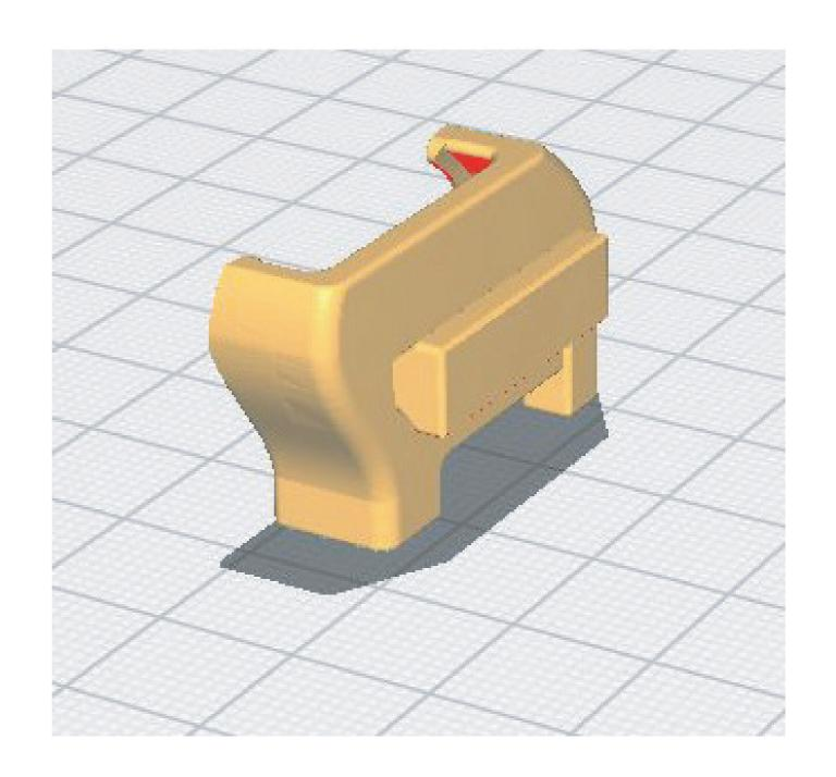
Positioning the model on the printing surface
