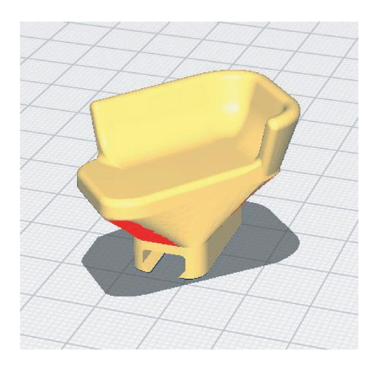
Positioning the model on the printing surface
