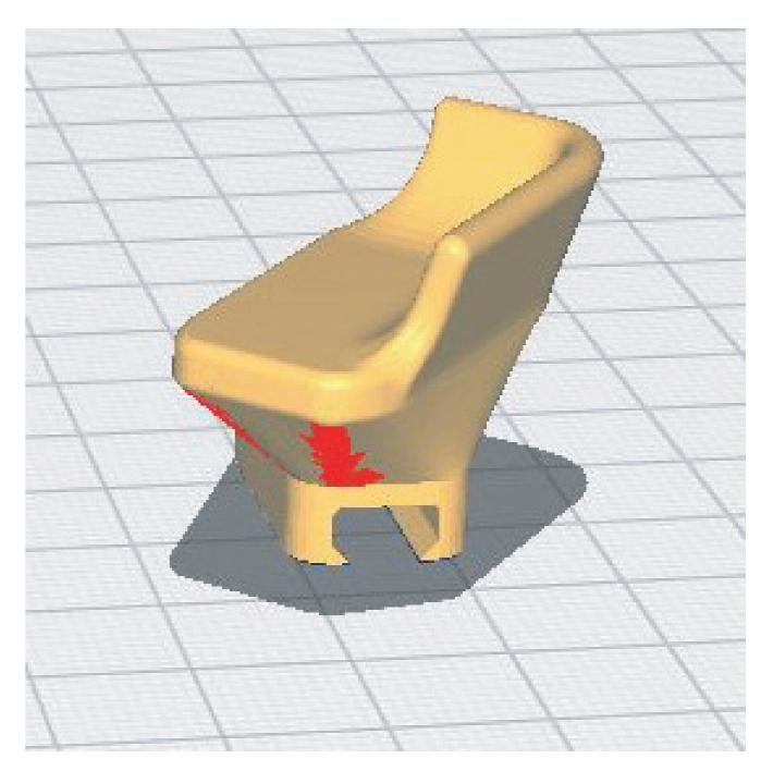
Positioning the model on the printing surface
