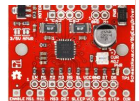
Figure 71: Big easy driver board
