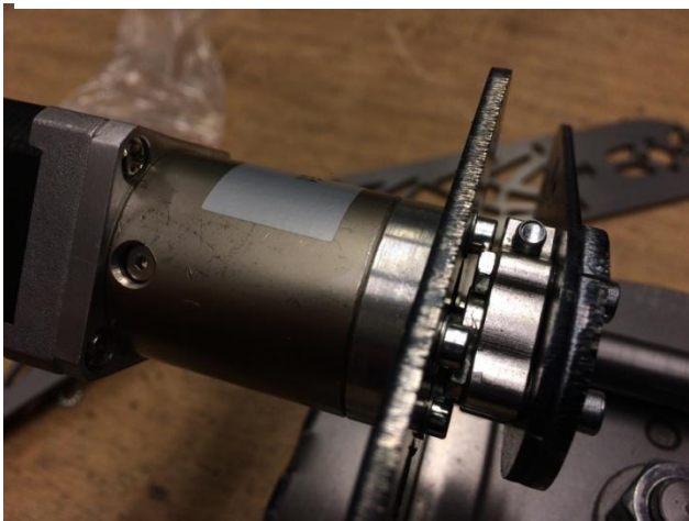
Figure 75: Motor bolts are hitting the bolts of the motor coupling.
