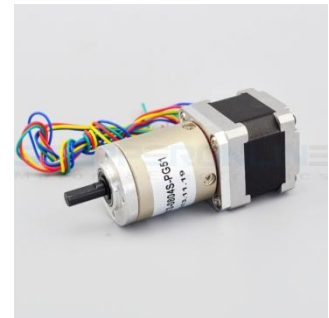
Figure 54: Stepper for the shoulder and elbow
