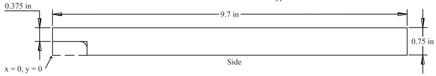
Cut in two places to remove a section to provide access to the motor mounting screws. Make a 0.375" deep cut at 0.95" on the x axis, and a 0.95" deep cut at 0.375" on the y axis. Optional -- For a smoother radius, first drill a 3/8" hole through both sides of the arm, centered at x=0.76" and y= 0.19".
