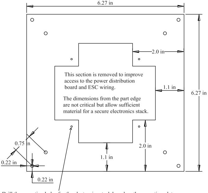
Drill the mounting holes for the electronics stack based on the mounting plate requirements and the hardware used to mount it.
