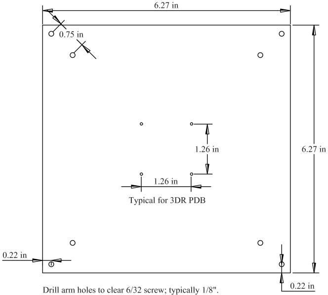
Drill arm holes to clear 6/32 screw; typically 1/8". Power Distribution Board holes are drilled to suit.
