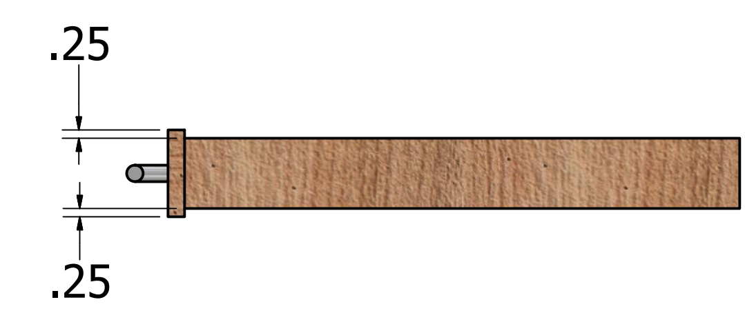
Drawer for 14.5" Wide x 2.75" High x 17.75" Deep Opening (Same Construction for Remaining Drawers)
