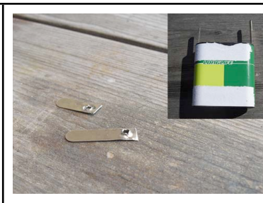
Now the electric inside, nothing complicated. I cut of the tongues of an old 4,5V battery, that would serve as a switch.
