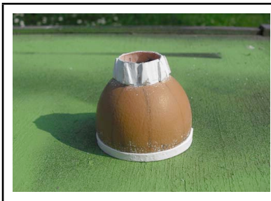
The ring is complete, with fitter (putty) and sandpapered, the ring, too, is ready to be painted.
