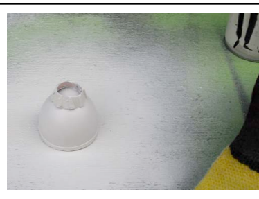
The first coating of the body, with a color that later turned out to be not white enough for the stickers. So it had to be sprayed again.
