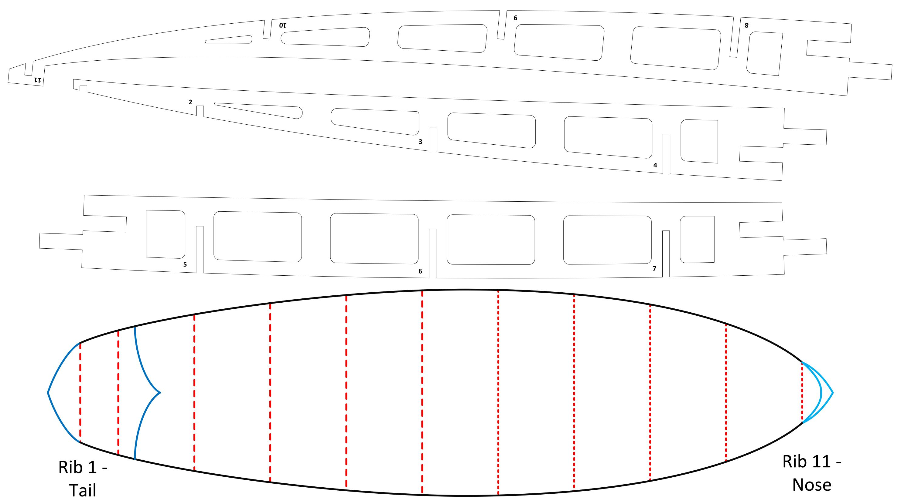
Build out the rails with all 11 ribs in. Then choose your tail shape and either cut it down for a fish, or extend for funboard. Add the noseblock and shape how you like it.
