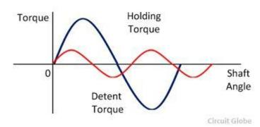
The torque which is caused by the motor when the rated current flow across the winding is known as the holding torque. Detent torque is beneficial for stepping the motor. It also resists the momentum of the moving rotor and the friction in the rotating components. Such type of torque is range from 5 to 20% of the holding torque.
