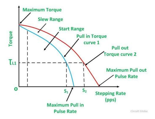
Similarly, the curve 2 represented by Red colour line is known as pullout torque characteristics. It shows the maximum stepping rate of the motor where it can run for the various values of load torque. But it cannot start, stop or reverse at this rate.
