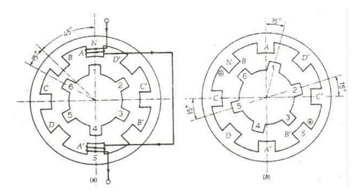
The opposite poles are connected in series forming a 4 phases. The rotor as 6 poles. Here I am considering only phase A to make the connection simple. When the coil AA' is excited the rotor teeth 1 and 4 are aligned
