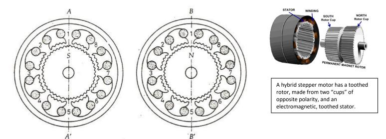
The stator has 8 poles, each of which has one coil and S number of teeth. There are 40 poles on the stator, and each end cap has 50 teeth. As the stator and rotor teeth are 40 and 50 respectively, the step angle is
