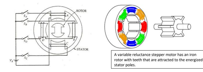
The four phases A, B, C and D are connected to the DC source with the help of a semiconductor, switches  $S_A$ ,  $S_B$ ,  $S_C$  and  $S_D$  respectively as shown in the above figure. The phase windings of the stator are energized in the sequence A, B, C, D, A. The rotor aligns itself with the axis of phase A as the winding A is energized. The rotor is stable in this position and cannot move until phase A is de-energized.
