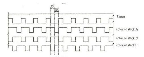
Similarly, now phase B is de-energized, and phase C is excited. The rotor moves another step of 1/3 of the pole pitch in the anticlockwise direction. Again, another change in the excitation of the rotor takes place, and the stator and rotor teeth align it with stack A. However, during this whole process (A - B - C - A) the rotor has moved one rotor tooth pitch.
