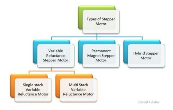
There are three types of stepping motor based on the rotor arrangements. They are as follows:-
