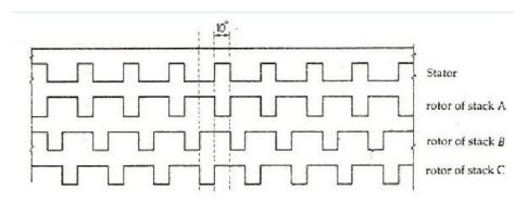
When phase A is de-energized, and phase B is excited, rotor teeth of the stack B are aligned with the stator teeth. The rotor movement is about 10 degrees in the anticlockwise direction. The motor moves one step which is equal to ½ of the pole pitch due to change of excitation from stack A to stack B. The figure below shows the position of the stator and rotor teeth when the phase B is excited.
