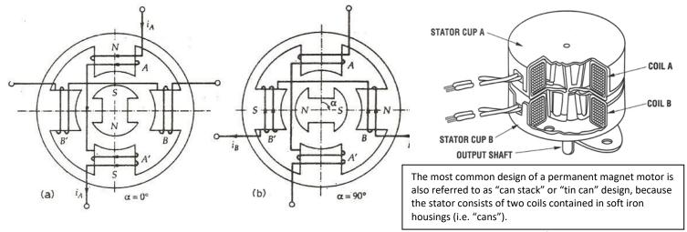
In figure (a) the current flows start to the end of phase A. The phase winding is denoted by  $A^+$  and the current by  $i^+_A$ . The figure shows the condition when the phase winding is excited with the current  $i^+_A$ . The south pole of the rotor is attracted by the stator phase A. Thus, the magnetic axis of the stator and rotor coincide and  $\alpha = 0^\circ$
