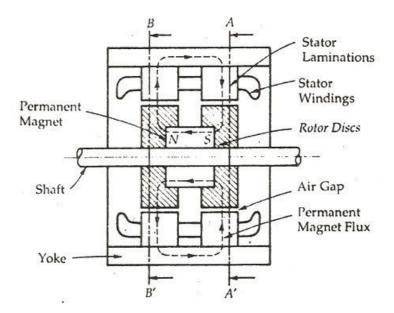
At both the end of the axial magnet the end caps are provided, which contains an equal number of teeth which are magnetized by the magnet. The figure of the cross section of the two end caps of the rotor is shown below.
