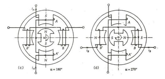
In the above figure (d), the current flows from end to starting point of phase B. The current is represented by  $i_B^-$  and the winding by  $B^-$ . Phase A carries no current and the phase B is excited. The rotor again moves further 90° and the value of  $\alpha = 270^\circ$
