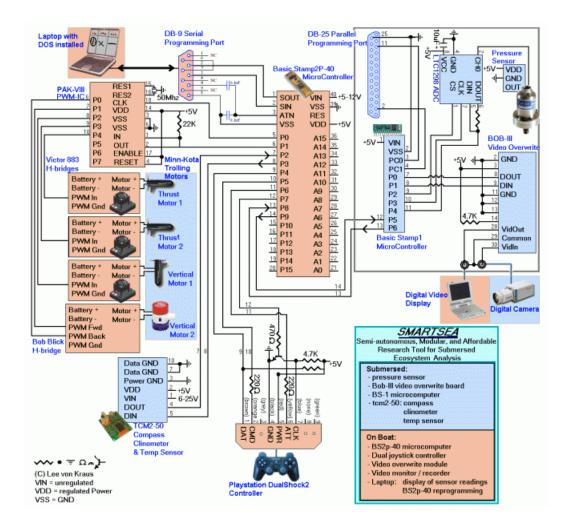
**Figure 1:** a circuit diagram showing the entire SMARTSEA electronics system. In the upper right is the video overwrite module (contains BOB-III, pressure sensor, ADC, and Basic Stamp1). In the center is the Basic Stamp 2p-40 microcontroller which serves as the middle man between the sensors, controller, laptop, and motors.
