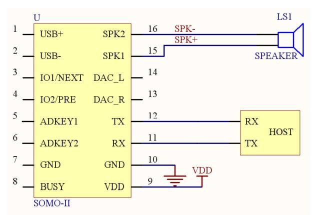
This example schematic shows a simple Serial connection to an external Host such as a 3.3V Microcontroller. It also shows the connections for an external speaker.
