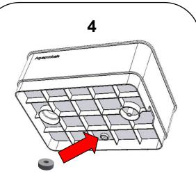
Wet the Gasket and then insert it into the underside of the Grow Bed where shown.
