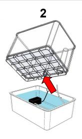
Insert the free end of the Hose into the underside of the Fish Tank Water Pipe until firm.
