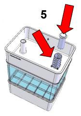
Place the Grow Bed on top of the Fish Tank. Insert the feet of the Shroud into the notches provided in the Grow Bed and then insert the Cap into the Shroud.
