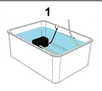
Place the Base on a level surface and fill with water to the level of the "FILL TO HERE" line. **DO NOT OVERFILL.** Push one end of the Hose onto the Pump outlet. Submerse the Pump with the electrical cable laid through the cut-out in the rear.
