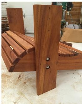
**3**-Install Top back support (#6) using 4- 2" screws while centering the 2 rear legs (#5) on screw holes. The front of the rear legs should be flush with front of the top back support
