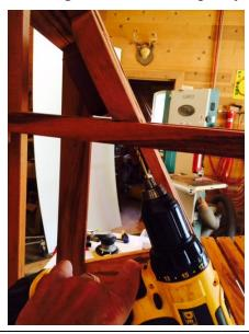
**18-** Predrill and install 4- 2 " screws thru bottom rear seat slat (#3) and into the fangs or the skull, while pulling the fangs tight to the brace.
