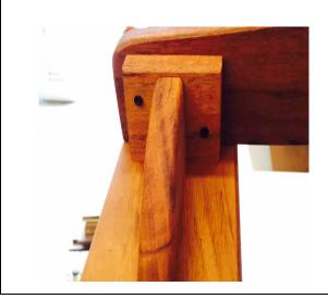
**8**-Attach the front of the arm to the front arm support by positioning it so there is approx 1/4" overhang to inside of the front leg. Pre-drill and install 3- 1 1/2" thru top plate of arm support and into the arm.
