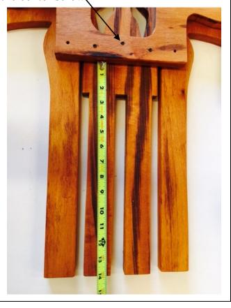
**12-**Use a square to be sure the mid brace is perpendicular and centered on the center skull piece #12. As shown here. Pre-drill and install the re-maining center screws.
