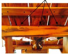
15-Lay and center the skull onto the chair. Pre-drill and install 1- 2" screw thru bottom of each arm into the skull, as shown. Making sure the skull is pulled tight to the upper back brace and sitting on each arm equally.
