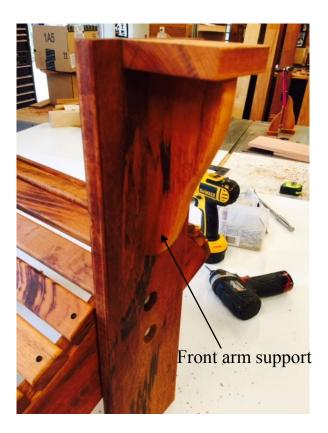
**6**-Make a mark on the outside of each back support upright at 21" from floor. This will be the top of the rear arm supports. Center the arm supports on the upright, pre-drill and fasten with 2- 1 1/2" screws.
