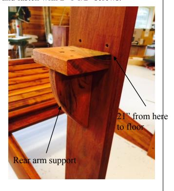
7-Lay the arm (#11) onto the arm supports and pre-drill and install 2-2" rear screw through back uprights (#5) while making sure the rear of the arm is flush/even with the rear edge of the upright.
