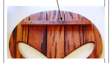
**16-**Install the skull mid brace (#18) on the underneath the top back support. Slide the brace up tight and centered under the back support. Pre-drill and install 6- 1 1/2" thru mid brace and into skull
