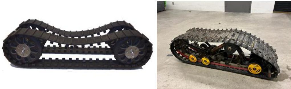
Figure 1: a) original two track system [3] b) mono-track system used.
