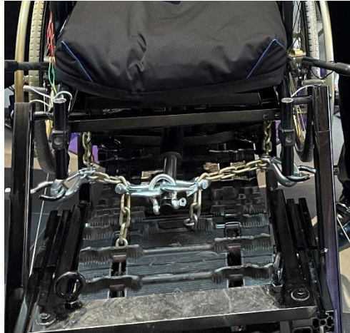
Figure 4: Chain connection to chassis.
