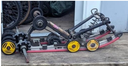
Figure 13: integrated suspension system and drive gear.
