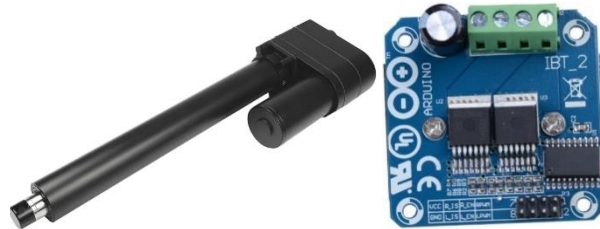
Figure 11: PA-17-8-2000-POT Actuator [7] and BTS 7960 Dual H-Bridge motor controller [8]
