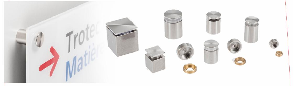
Stainless Steel Matt | Stand Offs Round, flat headed, left-hand thread Diameter: 15mm (0.59") Wall Distance: 15mm (0.59") Sign Thickness: 2-5mm (0.08"-0.2")
