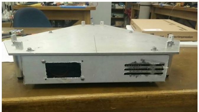
Figure 11: Electronics enclosure suspended under the platform base (incomplete).
