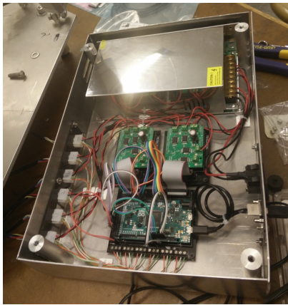
Figure 10: Finished electronics enclosure, front.
