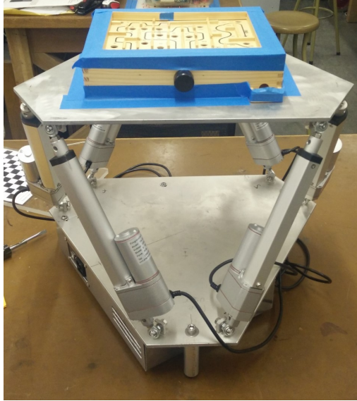
Figure 13: Platform with commercially available tilt maze, used for initial testing and feedback.
