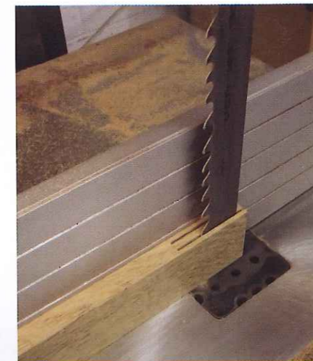
6 Cutting the tenon cheeks on the bandsaw
