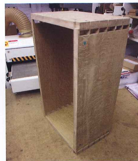
5 Partial assembly before adding any glue saves time. Don't forget to include the base
