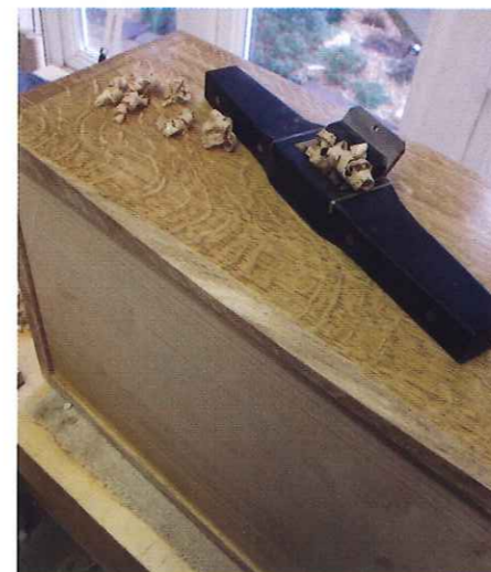
10 Cutting a tapered chamfer on the bottom edges of the box
