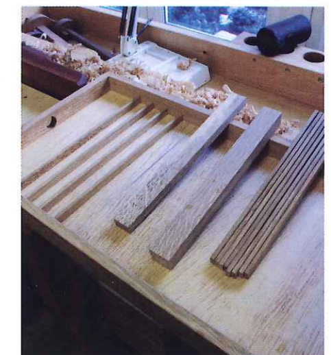
12 Fitting tray dividers using spacers and trimming on a shooting board
