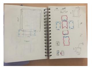
After creating the Illustrator file with me, Kathryn cut out the file to test it out and see if it had worked. She cut her version out with 1/8 inch thick plywood. She found that the two pieces on the back piece of the box was press fit when it wasn't supposed to be because the back piece needed to slide off in order to refill the teaholder with tea. She gave me the box and suggested to change the width of the two pieces so it would slide instead of press fitting together.
