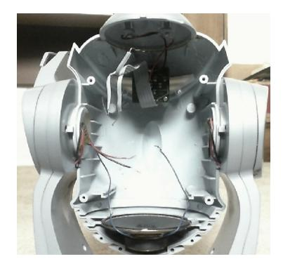
The red chest light remains. Also, you can see the speaker wires (blue) and motor wires on each side. I also used the wire already attached to the antenna on the robot's head to connect to the Minty Mote's receiver coil.
