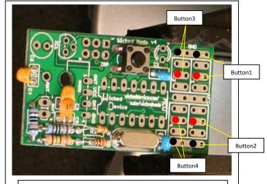
The picture above shows how to wire the 4 buttons to the receiver board of the Minty Mote.
