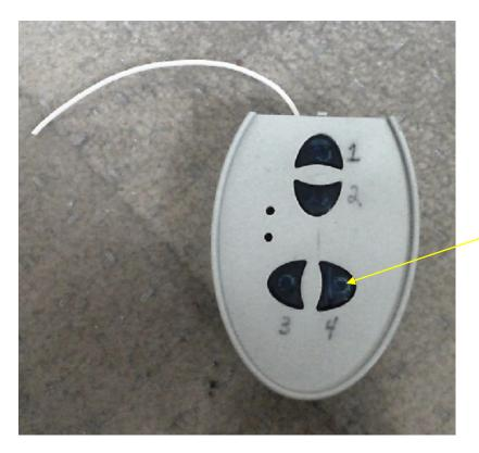
The Remote has a perf. board in it with 4 push buttons.
