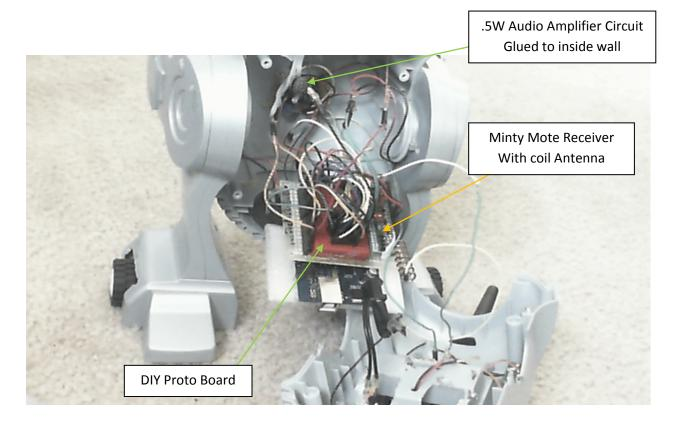
Here is all the circuitry that's inside the robot. The motors are driven by a LM293D H-Bridge. There is a tilt switch on the protoboard in the form of a ball switch which can be obtained from <a href="AdaFruit">AdaFruit</a>.
