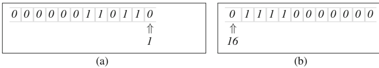
Fig. 5.17 The unary multiplication TM initial tape, a consists of two strings of ‘1’s the length of which represent the values. The TM starts in state one with the read/write head just to the right of the rightmost ‘1’. The unary multiplication TM final tape, b consists of one string of ‘1’s the length of which represents the value. The TM stops in state 16 with its read/write head just to the left of the leftmost ‘1’. a Initial tape. b Final tape
