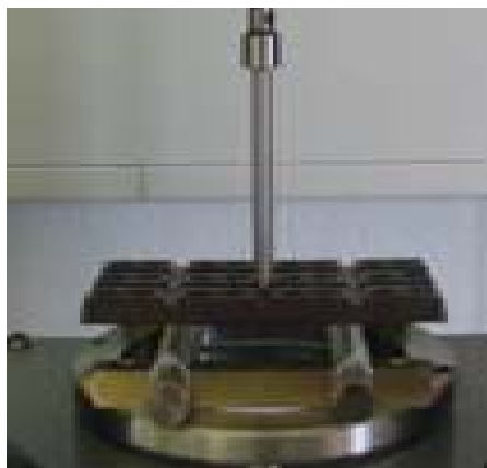
Fig. 3: Breaking test on a chocolate bar on the HAAKE MARS using the new bending geometry.
