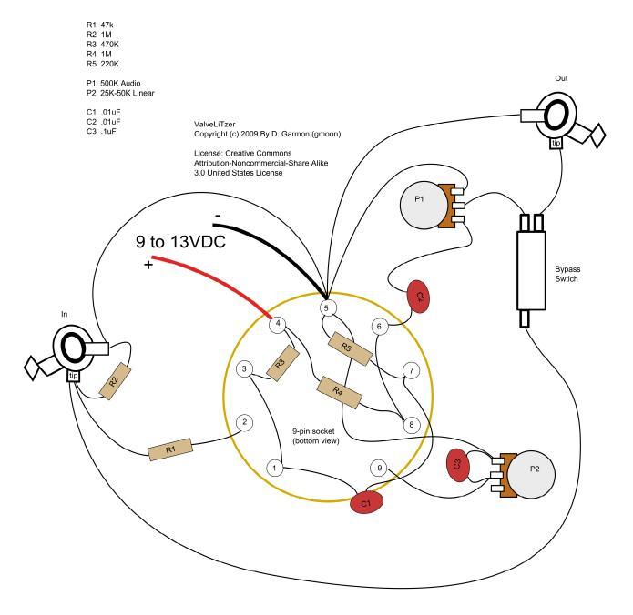
As wired, the bypass isn't a "true bypass," since some load is always appled at the input... A more complex bypass scheme can be used if desired.
