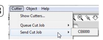
Once your design is ready, make sure the machine is on and your material is loaded. (Refer to machine set up handout.) Click Cutter>Send Cut Job>CE6000. "Cutters" menu will open on the right side of the screen. Click "Send to Cutter."
